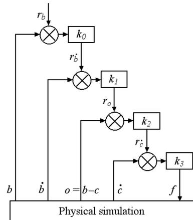
Figure 2: Control hierarchy for inverted pendulum
