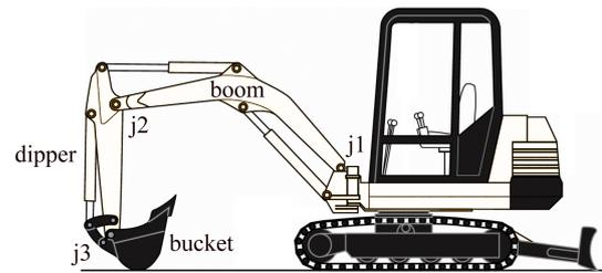
Figure 7: Backhoe excavator (JCB model 803)
