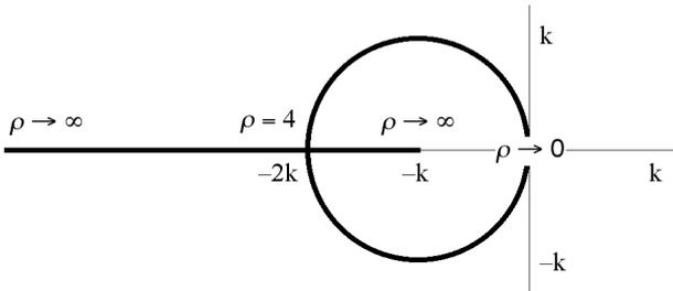
Figure 3: Root locus of two-level control system
